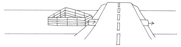
A simple pond leveling device (see below) can be an easy-to-build solution to flooding from beaver dams. A culvert pipe is installed in an intact beaver dam, and the inlet is sunk into the upstream beaver pond. A cage of heavy welded wire is constructed to prevent beaver from plugging the intake. The outlet end of the pipe can be set higher or lower in the dam depending on the desired level.
