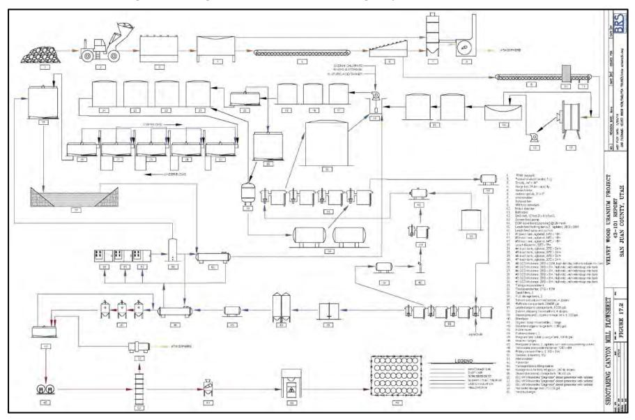
Figure 17.1 - Original Flowsheet for the Shootaring Canyon Uranium Circuit
