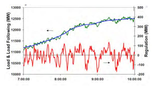
Figure ES-3. Regulation and load following during normal conditions.
