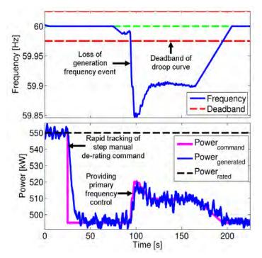
Figure ES-8. Field test data that shows the turbine tracking a step change in the de-rating command followed by PFC response to an under-frequency event.
