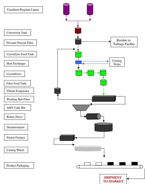
Figure 17.3 - Vanadium Purification and Precipitation Circuit, Page 2 of 2
