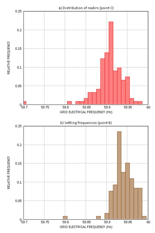
Figure ES-4. Distribution of low-frequency event data. Point C is the frequency nadir and point B is the settling frequency.
