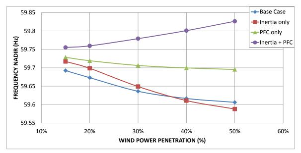
Figure ES-5. Impact of wind power controls on frequency nadir.
