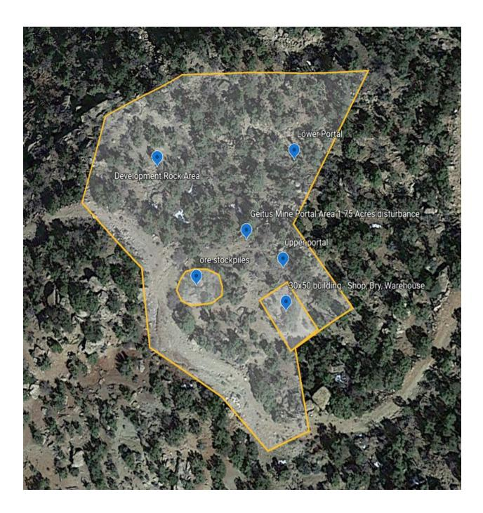
Figure 3- 4: Portal Site showing proposed surface facilities
