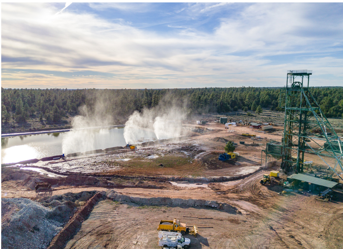
Landsharks next to the evaporation pond misting water into the air at Canyon Mine on March 15, 2017 to speed up evaporation. BLAKE MCCORD
