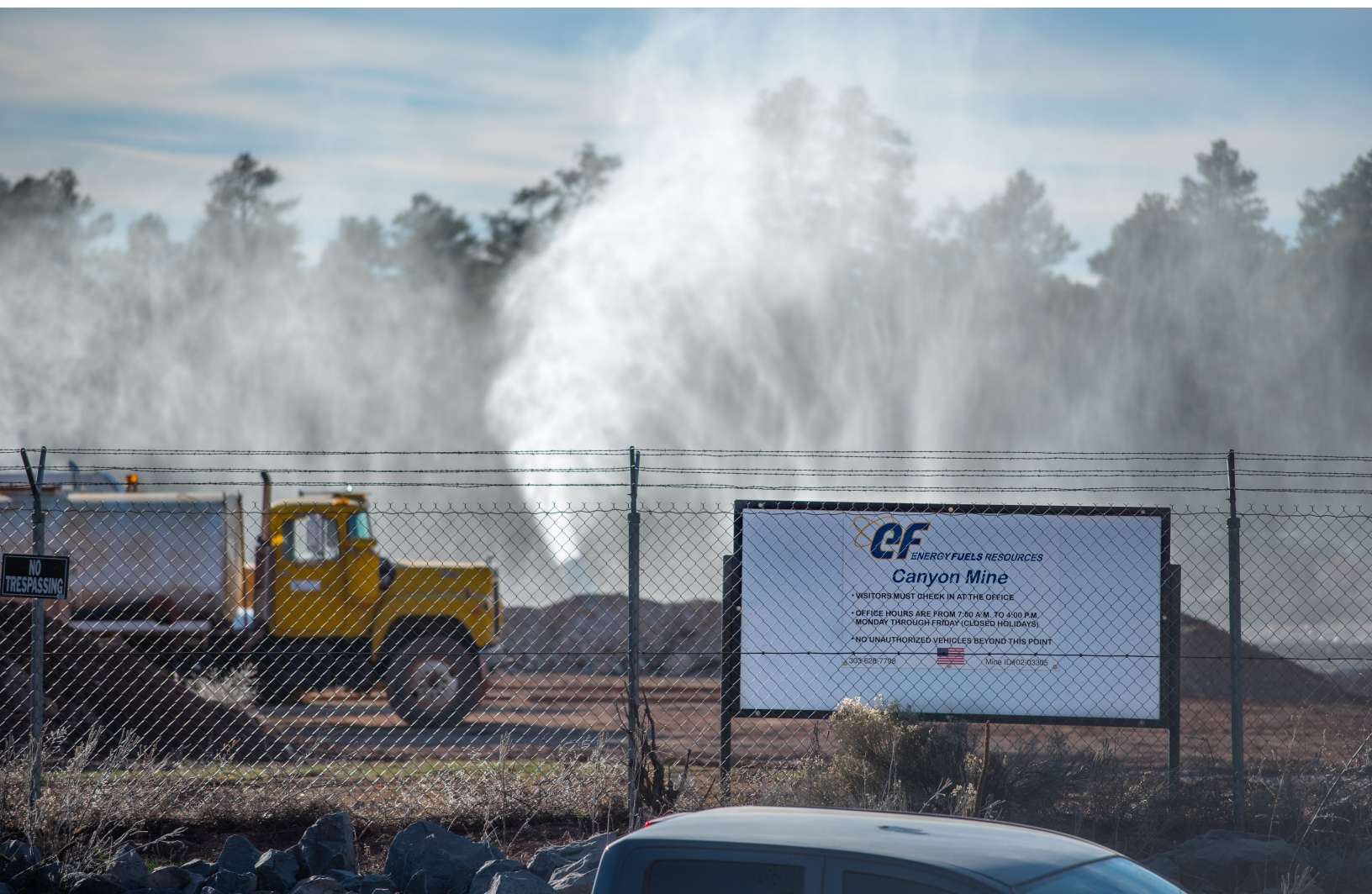
Energy Fuels Resources misting water into the air at Canyon Mine on March 15, 2017 to speed up evaporation. BLAKE MCCORD
